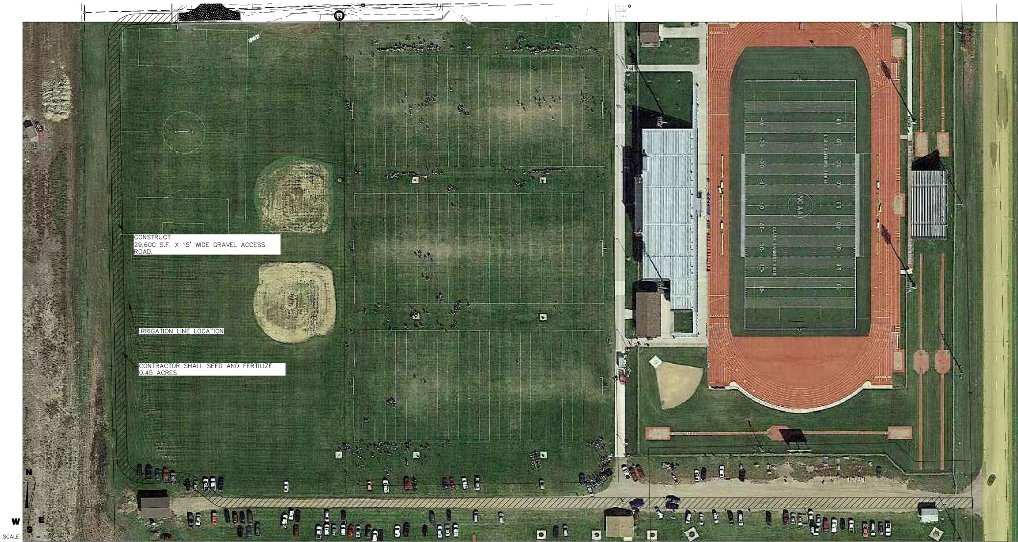
THE GRAVEL ACCESS ROAD SHALL BE CONSTRUCTED FIRST AND AT THE END OF THE PROJECT THE AREA SHALL BE RETURNED TO THE NATURAL STATE. GRAVEL FROM THE ROAD IS TO BE USED ON THE GRAVEL BUILDING PAD.
